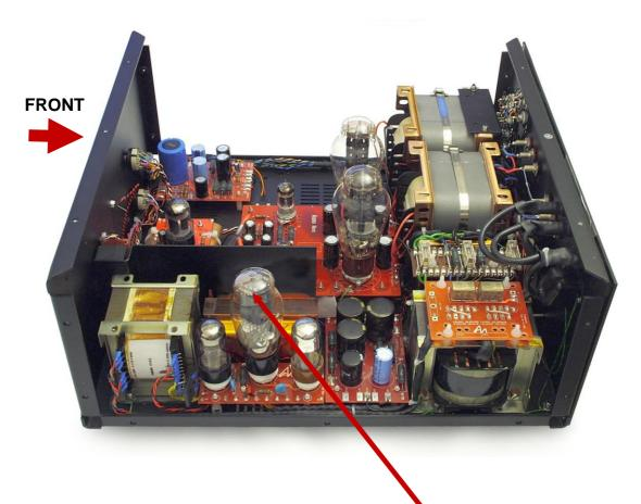
Looking from the front of the amplifier, insert the **5U4G** valve into the last empty socket located on the right, situated between two smaller valves. Locate the rib on the central pin of the valve and align with the valve base (it can only be inserted one way due to this locating rib) and with gentle but firm pressure insert the valve.
